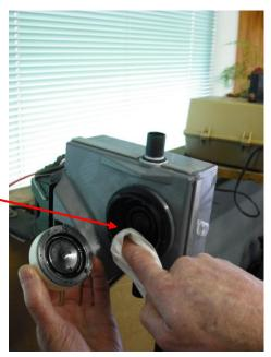
7. Clean both under the diaphragm on the front and the white body surface of the diaphragm.
