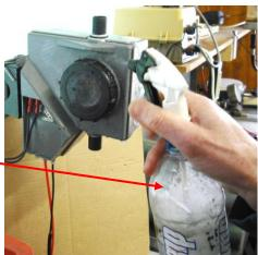
3. Divert the air from the sensor by pressing the start bulb to show bottom green light for STD model and on remote display for RD models.
