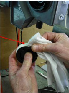
8. Fit diaphragm and tighten cap so that the index marks match up.
