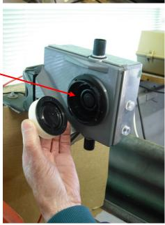
6. Use a damp clean cloth or tooth brush and clean the inside of sensor.
